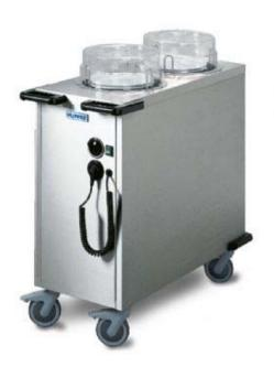
Plate stacker to receive round plates, Ø 190 to 260 mm, within 2 statically heated stacking tubes. Constant dispensing height by means of manually adjustable tension spring system.
